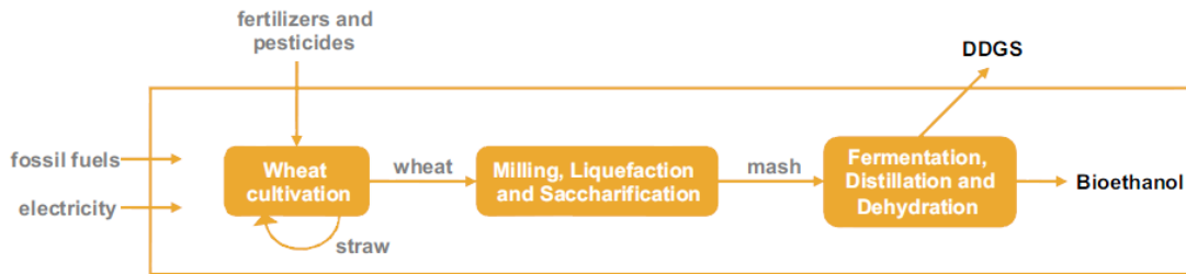
Flow chart illustrating the life-cycle chain (well-to-tank) of wheat-based bioethanol.
